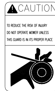
5. On the panel of mower deck and guard plate of LH&RH belt shield
